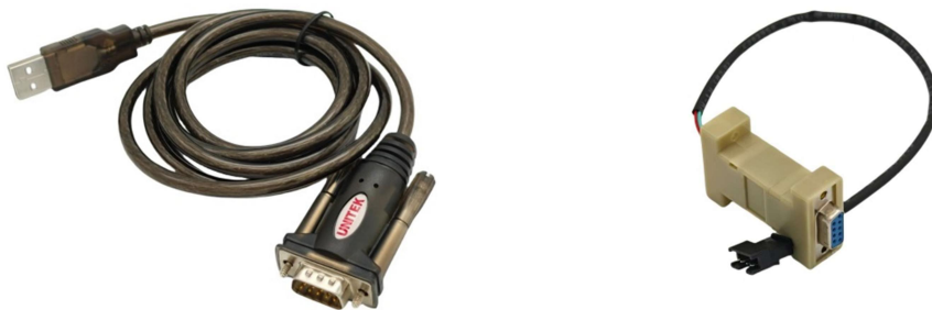
Figure 16: RS232-USB (left) and SM 4-Pin (right) adapter
