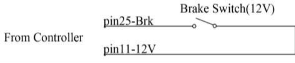
Figure 8: Wiring of brake switch(12V): 12V is provided by KLS-S controller on pin11
